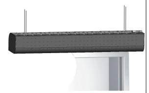
Before installing, check that the ceiling can bear the weight of the unit. Install according to the following figures.
