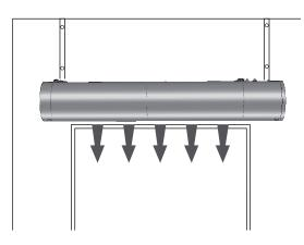
If there is a window above the door or another material preventing the installation on the brackets, the unit may be hanged from the ceiling with threaded rods, directly onto dowels (see below).
