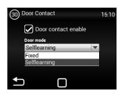
**Selflearning-** available only in automation and active function mode (Auto speed control), depending on the number of open doors it optimises the period in which the shutter is in operation, even when doors are closed.
