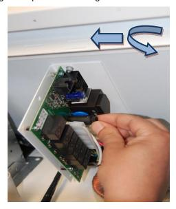
**PCB replacement:** Open the service panel and simply unscrew the power plate from the inside of the air curtain to remove it and make the necessary repairs.
