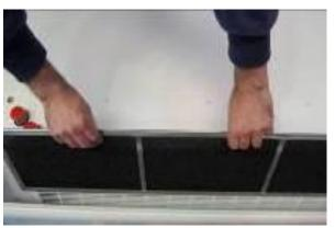
The inlet grille prevents the settling of dust and strange objects in the internal elements. It is recommended to check periodically that the inlet grille is free of any object that could interfere the air entrance (plastic bags, papers, etc.).
