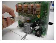
Unplug the two connectors of plate pressing the fluke.
