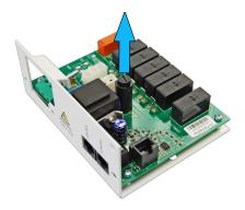
**Power board change:** open the service door and unscrew the power board from the inside of the air curtain to remove the plate and carry out the necessary repair.
