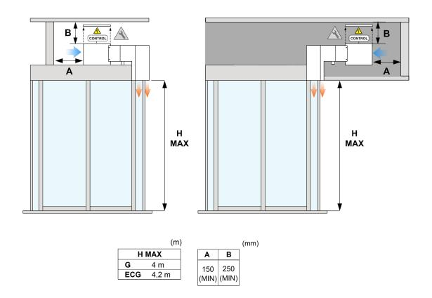
H MAX. Maximum recommended range, MIN. Recommended minimum distance
