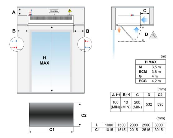
H MAX. Maximum recommended range, MIN. Recommended minimum distance
