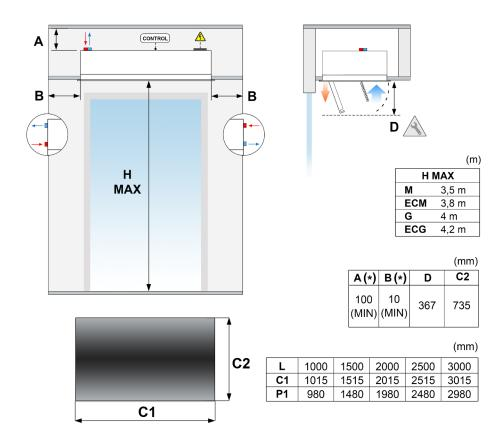
H MAX. Maximum recommended range, MIN. Recommended minimum distance
