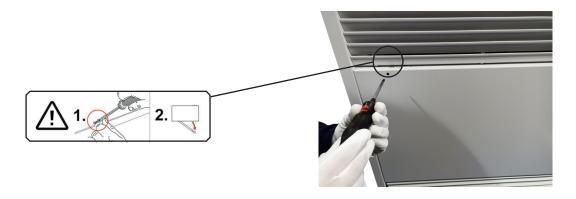
3. Raise the grate of the service door to be able to open the panel. Open the panel, being careful not to drop the grate of the service door. Once the service panel grille is closed with the service door open, open the service door fully with both hands
