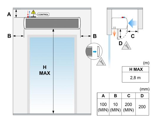
H MAX. Maximum recommended range, MIN. Recommended minimum distance. The minimum recommended distance between the suction grille and any obstacle is 200 mm (Dimension C) Dimension D: service opening distance.
