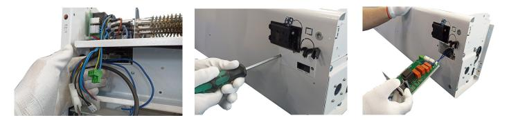
**Change fuse:** remove the pcb from the curtain for better maneuverability, remove the fuse protection casing and remove the fuse by hand or with the help of a screwdriver. Proceed to make the replacement and follow the reverse process to leave the curtain functional.
