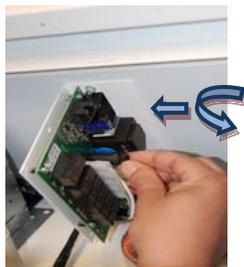
**PCB replacement:** Open the service panel and simply unscrew the power plate from the inside of the air curtain to remove it and make the necessary repairs.
