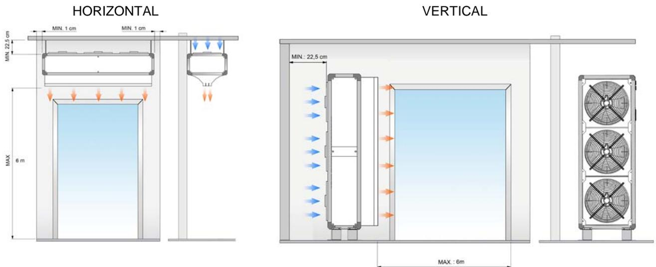
MAX. Maximum recommended height, MIN. Minimum recommended distance
