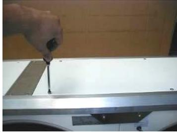
2.- Remove the panel carefully. If available, use a sucker, if not a screwdriver will do.
