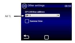
Ad 1) – Sets the CAN address of the control panel so up to 2 control panels may be connected to the MASTER regulator
